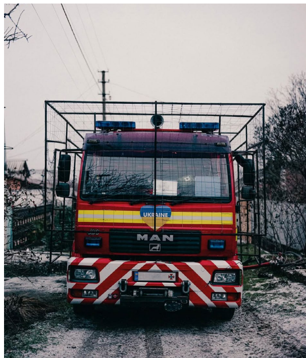
An SES vehicle in Nikopol with slat armor for protection from drones, December 2025. Source: Edward Matthews. 300
